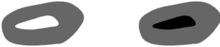
Fig. 19a: Cut a hole in an area object, Fig. 19b: Fill in a hole
