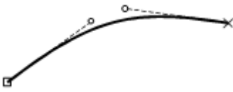
Fig. 13: Selected Bézier curves displaying the starting point, vertex, tangents and endpoint
